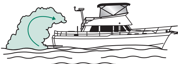
Figure 3. When protective weather coverings are in place, engine or generator exhaust from your yacht, while docked and/or running, can cause excessive accumulation of Carbon Monoxide gas within the cabin and cockpit areas of your yacht. Always provide adequate ventilation when the weather coverings are in place and either the engine or generator are running.
