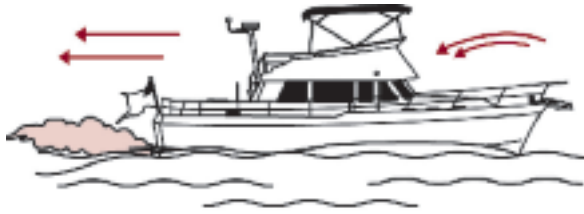
Figure 4. Engine or generator exhaust from your yacht while underway and operating with a high bow angle can cause excessive accumulation of Carbon Monoxide gas within the cabin and cockpit areas of your yacht. Always provide adequate ventilation and redistribute the load to lower the bow angle.
