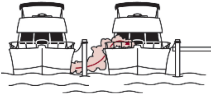
Figure 2. Engine and generator exhaust from other vessels alongside your yacht, while docked or anchored, can cause excessive accumulation of Carbon Monoxide gas within the cabin and cockpit areas of your yacht. Be alert for exhaust from other vessels.
