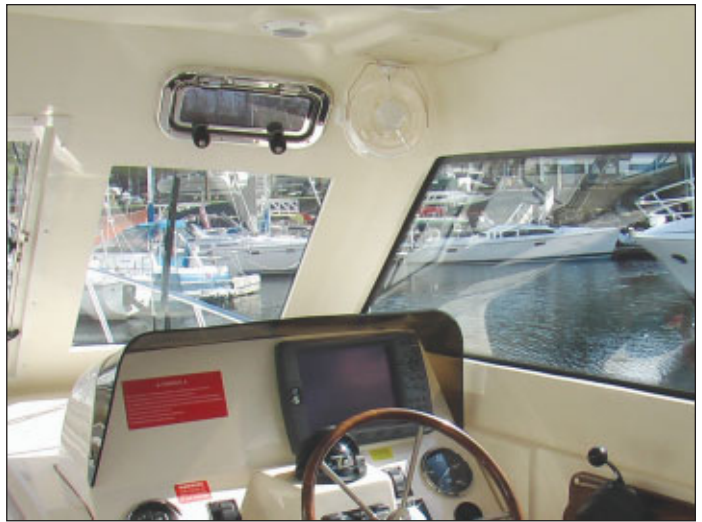
The whole dash, including the wheel, is hinged. Note the fan and small port up high.
