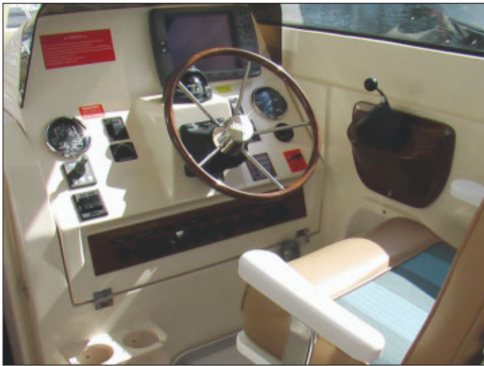
The whole dash, including the wheel, is hinged. Note the fan and small port up high.
